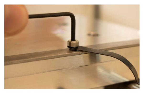
It can be helpful to move the Y Carriage to a position that allows for the Probing Clip to hang below the surface of the spoil board when installing it.
