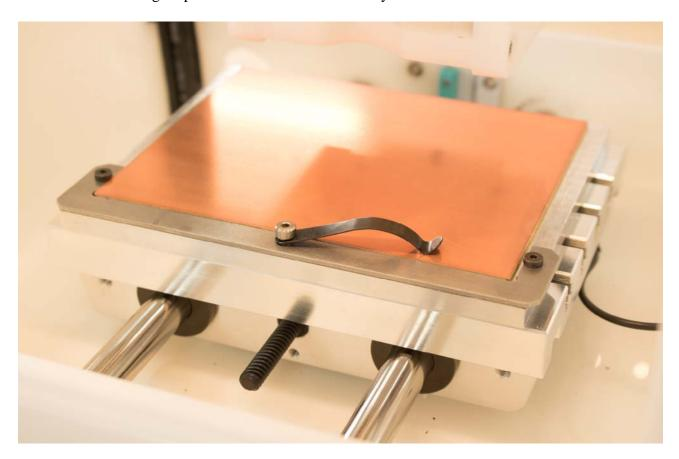
The clip works by electrically connecting the PCB material with the bed.
