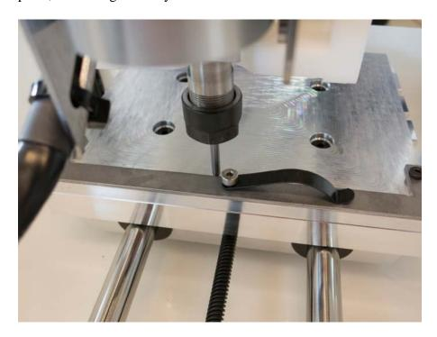
When locating the alignment bracket, the bracket edge is probed just to the left of the center mounting bolt. If the clip is installed in the center mounting hole, leave the clip resting to the right of the hole to avoid interfering with the bracket locating process.
