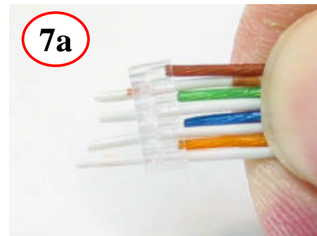
Trim Even wires (2, 4, 6, & 8) even with bottom of Management Bar and insert into Even row
