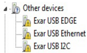
Figure 4: Enumeration of USB downstream ports
