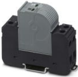
Pluggable type 2 arrester (surge arrester) for 1-phase current supply networks with separate N and PE (3-conductor system: L1, N, PE), with remote indication contact. Overall width: 24 mm.
