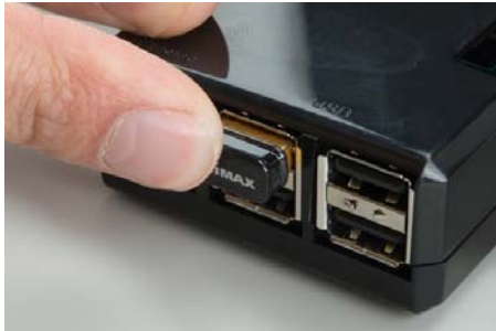
Inserting the Edimax wireless dongle. In this picture, the Edimax is fully seated.
