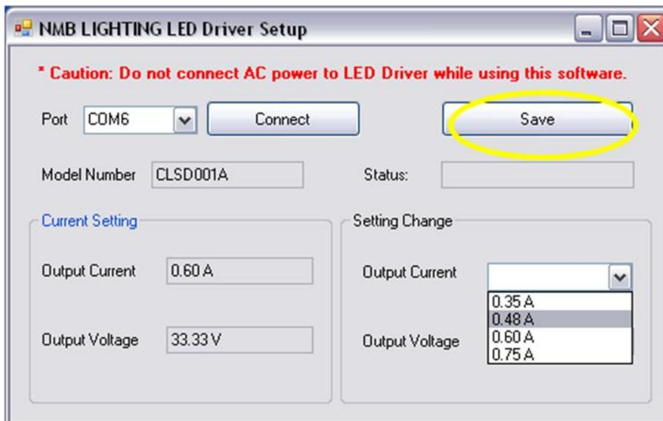
**Step 11:** The Status on the screen will change to Save Complete, and you have now programmed the output current to 0.48 A.
