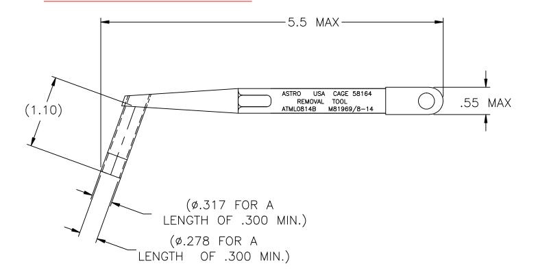
3. WITH TIPS CLOSED AROUND A .2770 +.0000/-.0002  $\phi$  PIN, MAX GAP BETWEEN TIPS TO BE .002.
