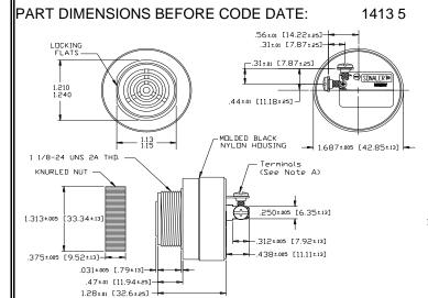
NOTE A: TERMINALS-.032 BRASS TIN PLATED, TAPPED FOR #6-32 SCREW. TWD #6-32 NICKEL PLATED BRASS SCREWS INCLUBED. WILL ACCEPT 1/4\* QUICK CONNECT. NOTE B: MOUNTING- REMOVE BLACK PLASTIC NUT AND INSERT THREADED FRONT THROUGH 1.25' HOLE PUNCHED IN PANEL, IF DRIENTATION IS NEEDED, NOTE LOCKING FLATS ON DRAWING. SCREV NUT BACK ON. DO NOT DVERTIGHTEN.
