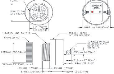
NOTE A: TERMINALS-.032 BRASS TIN PLATED, TAPPED FOR #6-32 SCREW. TWO #6-32 NICKEL PLATED BRASS SCREWS INCLUDED. WILL ACCEPT 1/4' QUICK CONNECT. NOTE B: MOUNTING- REMOVE BLACK PLASTIC NUT AND INSERT THREADED FRONT THREUGH 1.25' HOLE PUNCHED IN PANEL, IF DRIENTATION IS NEEDED, NOTE LOCKING FLATS ON DRAWING. SCREW NUT BACK ON. DO NOT OVERTIGHTEN.
