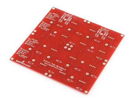
**Description:** This a simple breakout board for the button pads. Each LED and button is brought out to the side connectors. The connectors are soldered to the back side of the PCB. We recommend trimming the connector leads on the button side as short as possible to reduce the deflection of the pad.
